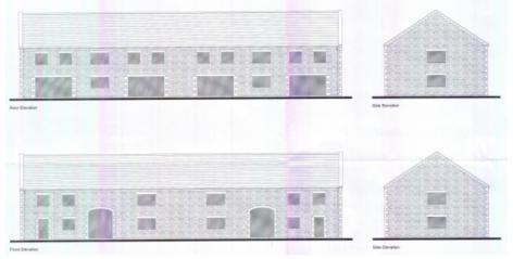
The elevation plan drawings of the former barn are not consistent and offer conflicting heights as to how much that the demolished barn was dug into the ground, varying from 1m to 1.7m on the north and south elevations. On the western elevation (the same elevation the above historic photograph illustrates) there is a constant 3.4m from ground level to the eaves. Rather than delay matters further requesting the agent to correct such anomalies they are recorded here for members to duly note.
